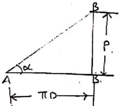
The height of the plane BC is the distance moved axially in one revolution of the screw in its nut, i.e. pitch ( $P$ ). The base of the plane (AB) is circumference of the thread at the mean radius, i.e.,  $\pi D$ , where  $D$  is mean thread diameter.
