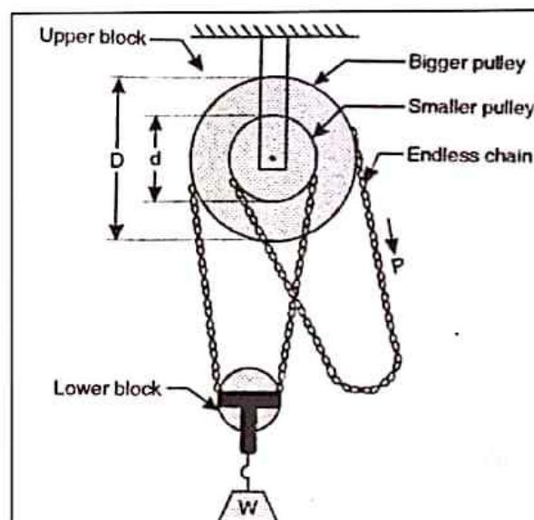
An endless chain passes over the bigger and pulley and single pulley in lower block as shown in the figure.
