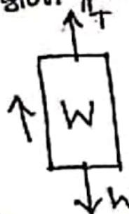
lift is moving upward.
