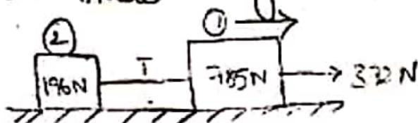
$$W_1 = 785\text{N}, W_2 = 196\text{N}, P = 392\text{N}, \mu = 0.3, a = ?$$
