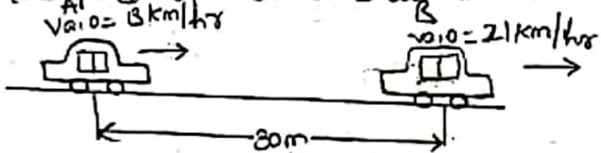
Sol:- Car A overtakes car B after  $t$  seconds, at a distance  $x$  metres from its start.  $x$  metres from its start
