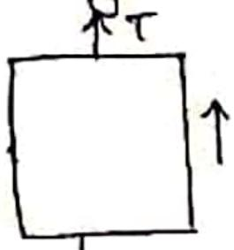
$$\begin{aligned}T &= w + ma \\&= 500 + 50 \cdot 9.77 \times 1.225 \\&= 562.496 \text{ N}\end{aligned}$$
