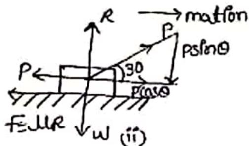
A body is resting on rough horizontal plane required a pull of 82N inclined at  $30^\circ$  to the done. Just move it. It was found that push of 100N in clined at  $30^\circ$  to the plane just moved the body. Determine weight of the body and the coefficient of friction.
