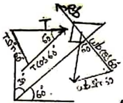
Resolving force normal to the inclined plane.
