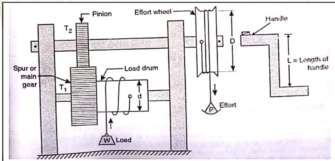
This machine consists of mainly the larger gear wheel known as Spur or main gear and smaller gear known as pinion. Spur or main gear is mounted rigidly on the load drum or load axle and the spur is geared to the pinion which is further mounted rigidly on the shaft to which the effort wheel or handle is attached.
