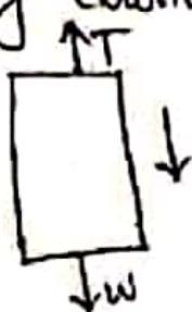
$$\begin{aligned}(w - T) &= ma \\T &= w - ma \\&= 500 - 50 \cdot 9.77 \times 1.225 \\&= 437.56 \text{ N}\end{aligned}$$
