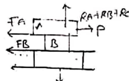
Two equal bodies A and B of weight  $W$  each are placed on rough inclined planes. The bodies are connected by light string. If  $\mu_a = k_1$  and  $\mu_b = k_2$  show that the bodies both on the point of motion when the plane is inclined at  $\tan^{-1}(k_2)$
