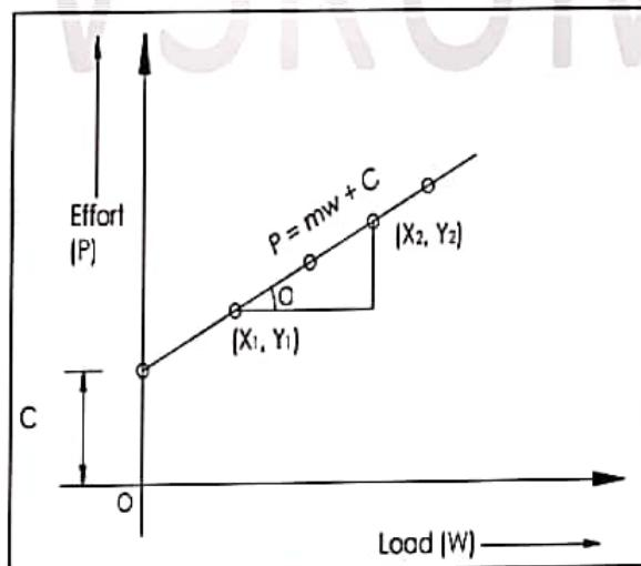
It has been observed that, the graph of load v/s effort is a straight line cuts the Y-axis giving the intercept 'C' which indicates the effort lost on friction, when no load is applied.
